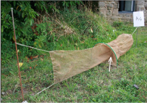
Fig. 1. Funnel trap used in the present study. The size of the entrance to the collecting chamber is 7 \times 7 cm (see arrow) and the paper sheet is at the A4 format.
