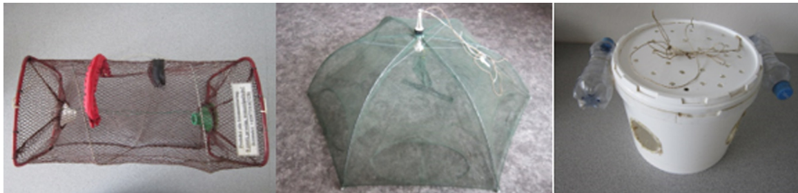
Fig. 1. Three types of traps used throughout this study. Prism shape (left), umbrella shape (middle) and Ortman's trap (right).
