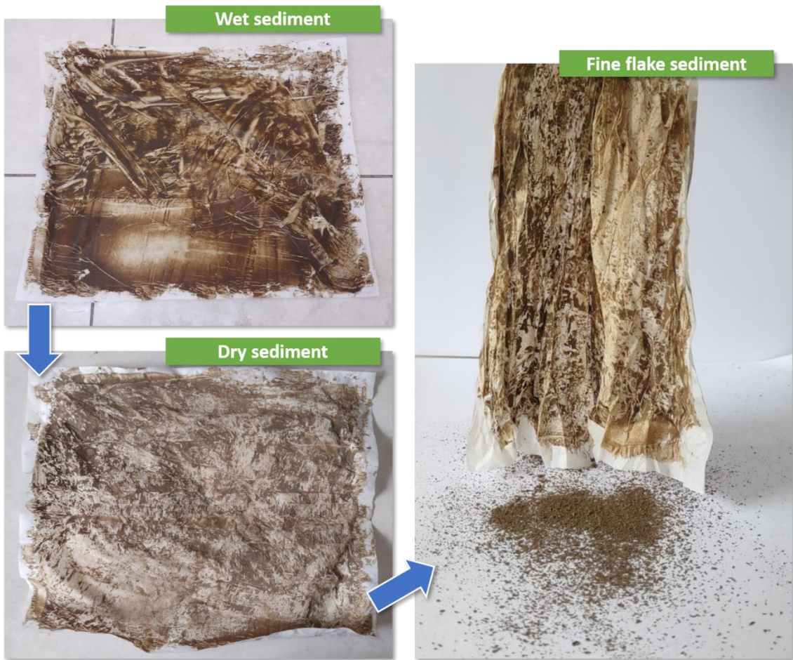
Figure S2. The visual aspect of the sediment sample during the drying process and formation of fine flake sediment following the proposed method.
