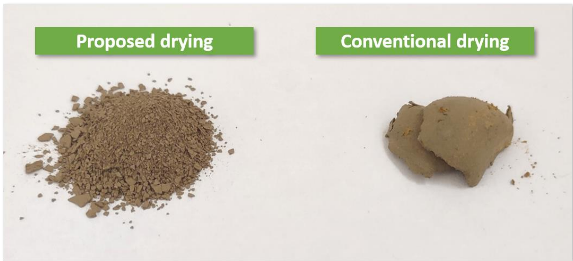
Figure S5: Sediment samples after the proposed drying process (left) and conventional drying process forming a solid mass (right).
